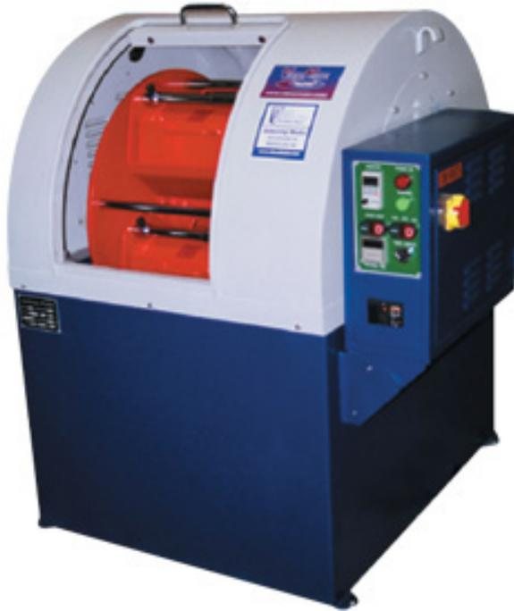
Standard CB Models 30, 60, 100 with horizontal barrels, variable speed, process timer, jog forward and reverse with quick disconnect.
