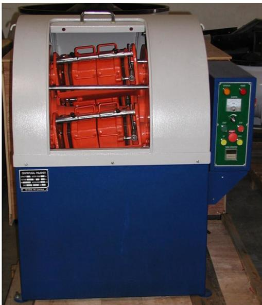
CBTB Models with angled barrels to produce "Figure 8" action for exceptional processing. Pictured are 8 half barrels to process several different parts at the same time.
